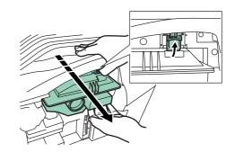
**NOTE:** Do not pull the toner container all the way as it can fall off and the toner spots the floor.
